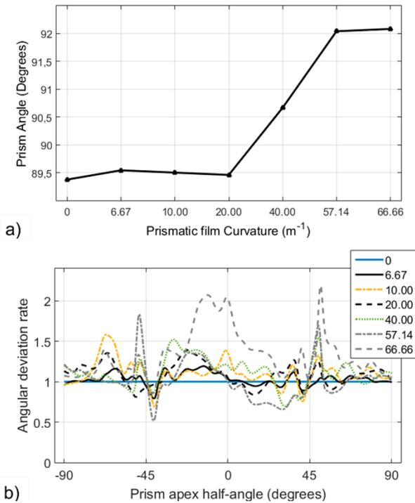
**Figure 4.** Angle  $\theta$  obtained by HT related with CPLG curvature. The graph legend shows curvatures evaluated in  $\text{m}^{-1}$ . Global changes in prismatic angle related with Hough peaks are shown in (a) and local changes in prism half-angle in (b).
