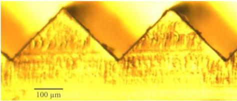
**Figure 1.** Image of a cross-section of the prism film used to analyze the contour (57X).
