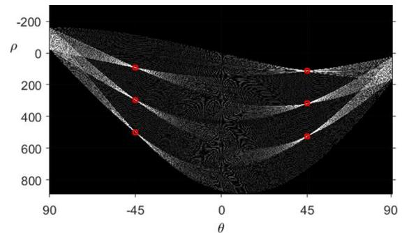
**Figure 3.** The HT of the three prisms image of prismatic film curvature of 20  $m^{-1}$  with Hough peak identified. The red square shows the peaks of data in the Hough matrix indicates  $\rho$  the perpendicular distance from the origin to
