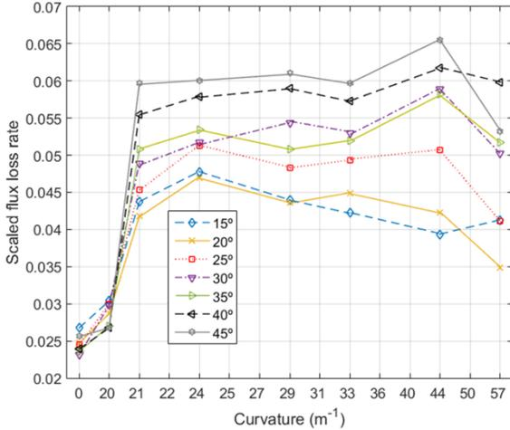
**Figure 6.** Light flux rate (rate of flux lost) scaled from 0 to 1.0 as a function of the curvature of a CPLG for several incidence angles. The graph legend shows incidence angles with regard to the prismatic film flat surface.
