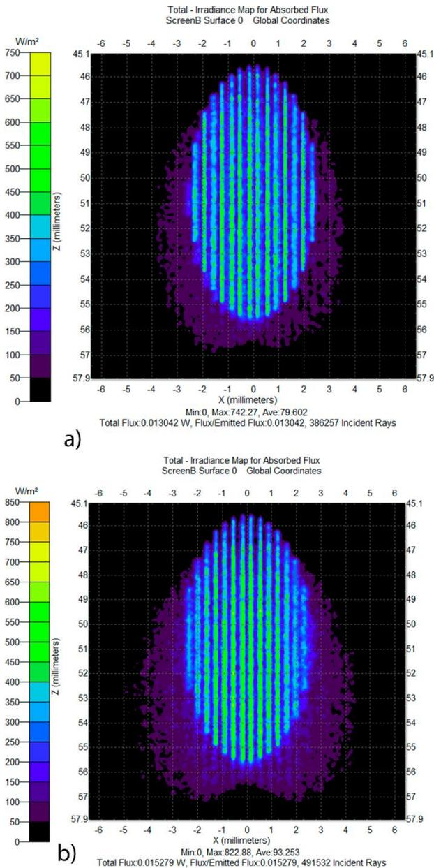
**Figure 7.** Flux loss rate obtained in tridimensional simulations of CPLG guides with curvatures of 8.00 (a) and 57.14 (b).
