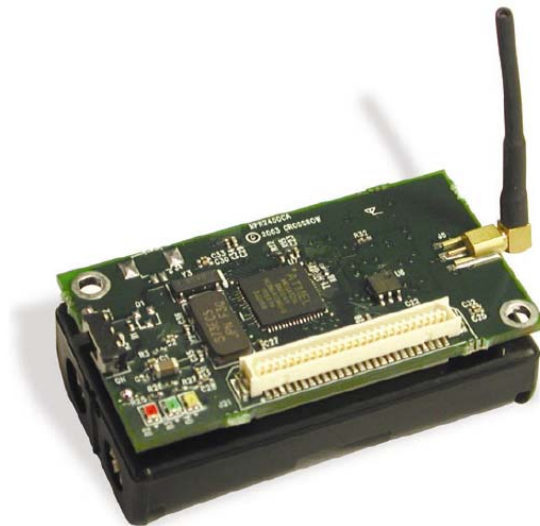
Figure 2.9. Photo of the MPR2400—MicaZ with standard antenna.
