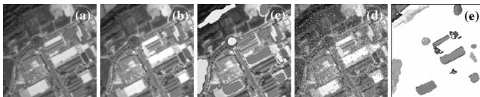
Fig. 4 a, b Urban area acquired by the IKONOS satellite at different times, c, d synthetic images obtained from b with artificial changes and noise with zero mean and variance 5.0; e changes obtained for the DSA method between the images (a) and (c)
