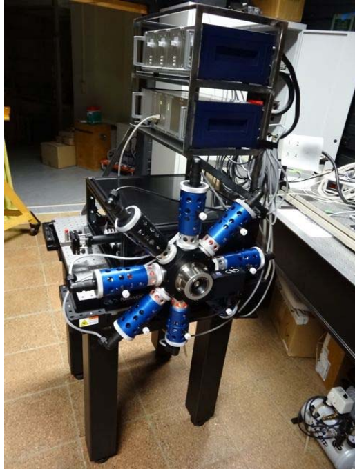
Figure 4. Calibration unit for the visible channel built by TLS. The housings for eight lamps in an octagonal arrangement are visible in the foreground of the picture on the left. In the right picture, the cover has been removed to show the optics feeding the calibration light into the fibers. External ports that can accept fibers from other calibration sources (e.g., etalons) are also available. The near-IR calibration unit is nearly identical.
