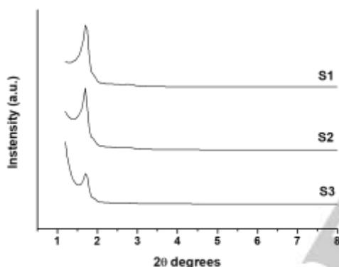
Figure 1. Powder X-ray diffraction patterns of solids **S1**, **S2** and **S3**.
